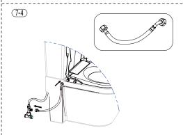
Make sure that flat seal kept in the flexible hose and then connect it to the  $\mathsf{T}$  shape joint.
