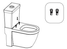
Put the plug nuts into the fastening hole on bowl.
