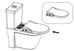
Insert the bidet seat onto the fixing plate and push it to the end. It is fixed while you hear a "click".
