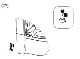
Make sure that flat seal kept in the T shape joint and then connect it to the inlet valve.
