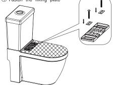
Refer to the figure above, place the fixing plate, washers and bolts onto the bowl in the opening of template.
