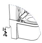
Connect the flexible hose onto the T shape joint
