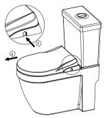
Keep the lid closed. Push the button on side and pull the bidet seat along the arrow shown in figure.
