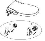
1.Pull out the old knob along the arrow direction as figure A.
