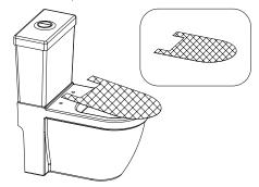
Place the template onto the bowl matching profiles between bidet seat and bowl.
